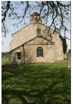
The west end of the **Nave** (left) is of good-quality coursed well-squared fawn sandstone, with some breaks in coursing where the re-used medieval fabric of the main wall abuts against the in-situ masonry of the buttresses at either end. The broad shallow-pitched gable has moulded kneelers and a square-section coping, and is capped by a Classical-styled bellcote that has a moulded round arch under an archivolt carried on raised pilasters.
